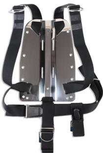
Dural backplate, thickness 3 mm with PA harness, stainless-steel D-rings and stoppers, stainless-steel buckle, crotch strap, buoy pocket and pocket with knife. Backplate is made of aluminium alloy resistant to salt water. Backplate is hard anodized. Edges bevelled on a NC cutter.
