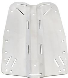
Stainless-steel backplate made of salt water resistant stainless-steel. Edges bevelled on a NC cutter, manually polished for perfect flattening of sharp edges, which could dilacerate the strap.
